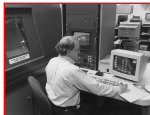
Yoder's well-equipped quality assurance lab with real time X-ray analysis
